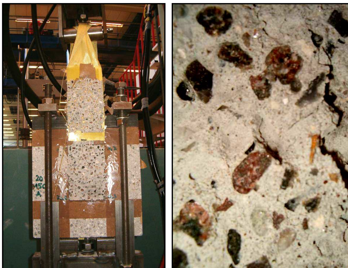
Figure 3.2.4 Example of the test setting – specimen 20 150 B – immediately after tension test, the structure of concrete after the failure
