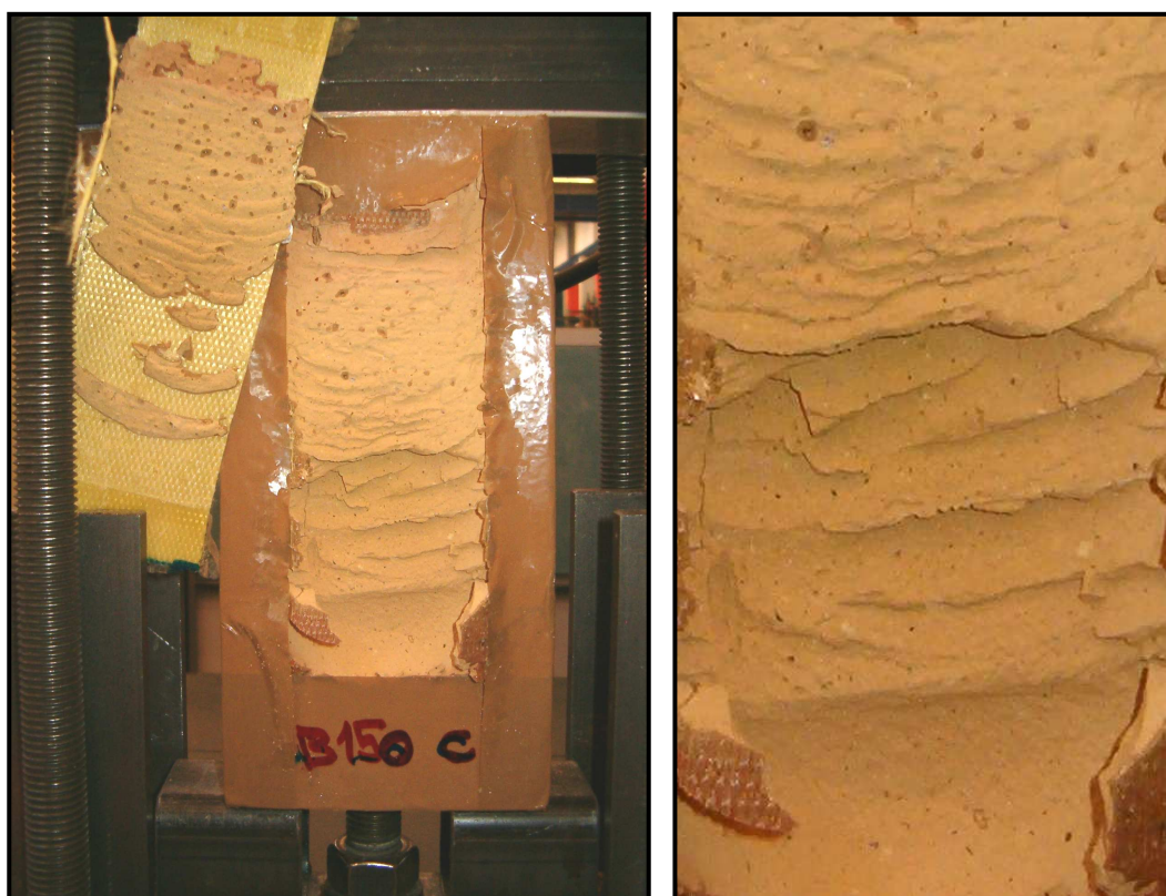
Figure 3.3.2 Example of the test setting – specimen B 150 C – immediately after tension test, the structure of brick after the failure
